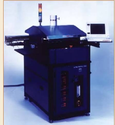
Sikama Ultra Profile 2000 System for BGA strip sphere soldering with small 48" x 38" footprint.
